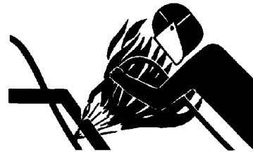
Heating Near Pressurized Fluid Lines
