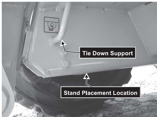
Fig. 2-13 View of the stand placement and tie down support locations.
