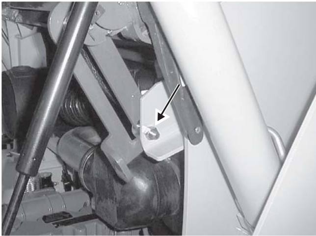
Fig. 2-7 Location of the self-actuating lock mechanism.
