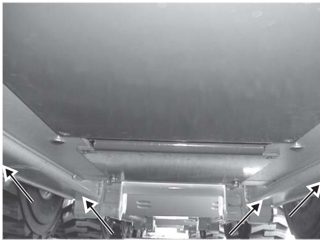
Fig. 2-14 Locations underneath the skid loader to position stands or blocks at the front and rear. (View is from the rear of the loader.)
